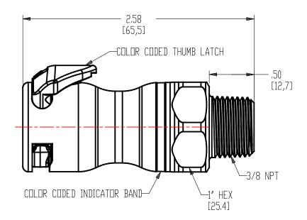
Description: 3/8" NPT Valved In-Line Liquid Cooling Body, Cool Blue
