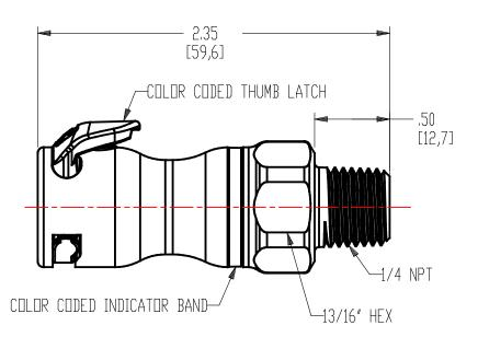
Description: 1/4" NPT Valved In-Line Liquid Cooling Body, Cool Blue
